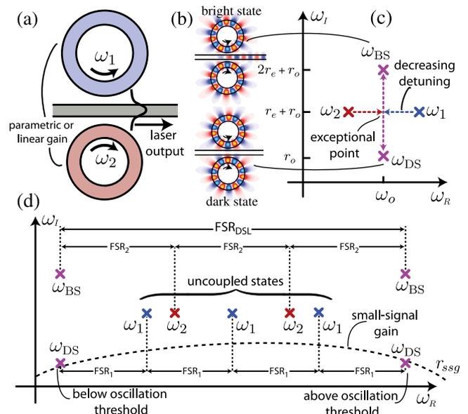
Fig. 1. (a) Proposed laser resonator geometry enabling far-field interference at the output coupler resulting in (b) a low- $Q$  (bright) state and high- $Q$  (dark) state with (c) eigenfrequency imaginary splitting at matched resonances to create (d) a broad Vernier-like FSR for ultrawide tuning.
