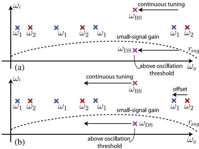
Fig. 4. Illustration of quasi-continuous tuning of the dark state laser. First (a) both rings are tuned across an FSR of the smaller ring (larger FSR). Then the laser can be turned off and reset to the start position [Fig. 1(d)]. (b) An offset then can be introduced to shift the  $Q$ -splitting to the previous location where both rings then can be continuously tuned across another FSR. The process then can be repeated across the gain bandwidth.
