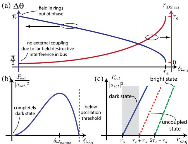
Fig. 3. (a) Phase difference between mode fields of each ring and resulting external coupling of dark state with detuning. (b) Dependence of tuning on output power for fixed  $r_e$ . (c) Threshold/slope efficiency curves as a function of small-signal gain (pumping), with the operating region of dark-state-only lasing shaded.
