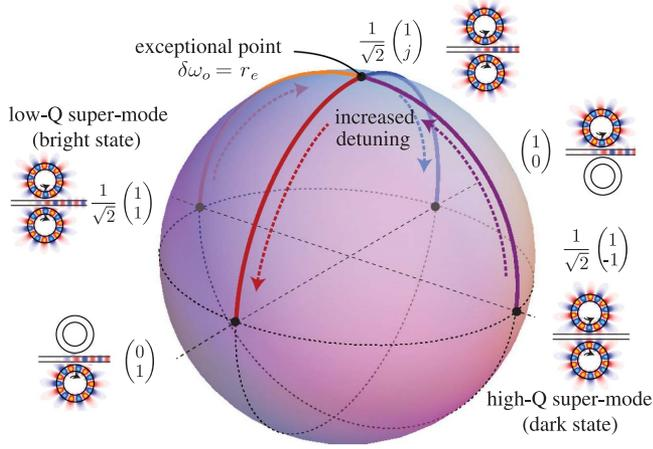
Fig. 2. Visualization of supermodes with detuning on a Poincaré (Bloch) sphere. For detuning less than the single-ring external coupling ( $\delta\omega_o < r_e$ ), the energy is equally distributed across both rings. At greater detuning, the supermodes approach the modes of the individual uncoupled rings.
