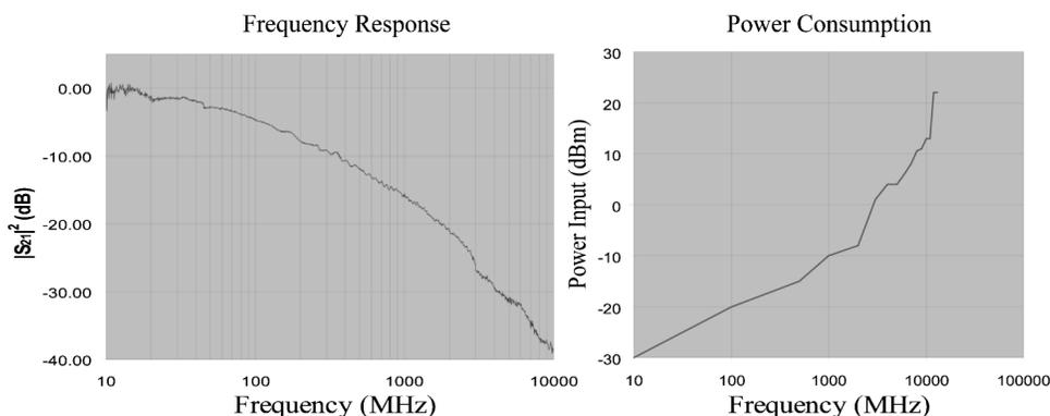
Fig. 7. (a) Frequency response of a 0.25 mm long MZ modulator operated in forward bias mode. (b) Power consumption of a 0.5 mm long MZ modulator under forward bias with 25% modulation depth.
