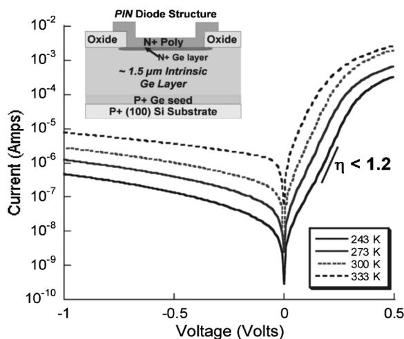
Fig. 8. I-V characteristics of a  $100 \mu\text{m} \times 100 \mu\text{m}$  diode as a function of temperature. The diode has an ideality factor less than 1.2 at 300 K with a perimeter dominated reverse leakage current of  $\sim 55 \text{ mA/cm}^2$  at -1 volt bias. Inset shows a schematic of a diode cross section.
