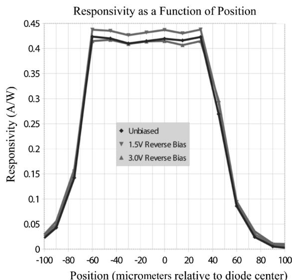
Fig. 9. Responsivity versus position for a  $100\ \mu\text{m} \times 100\ \mu\text{m}$  diode with no antireflective coating. A lensed fiber probe is translated across the surface of the detector to spatially resolve the responsivity.
