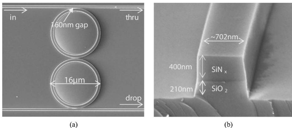
Fig. 1. (a) Top view of a second-order microring resonator filter. (b) Cross-section view of the bus waveguide showing smooth vertical sidewalls.
