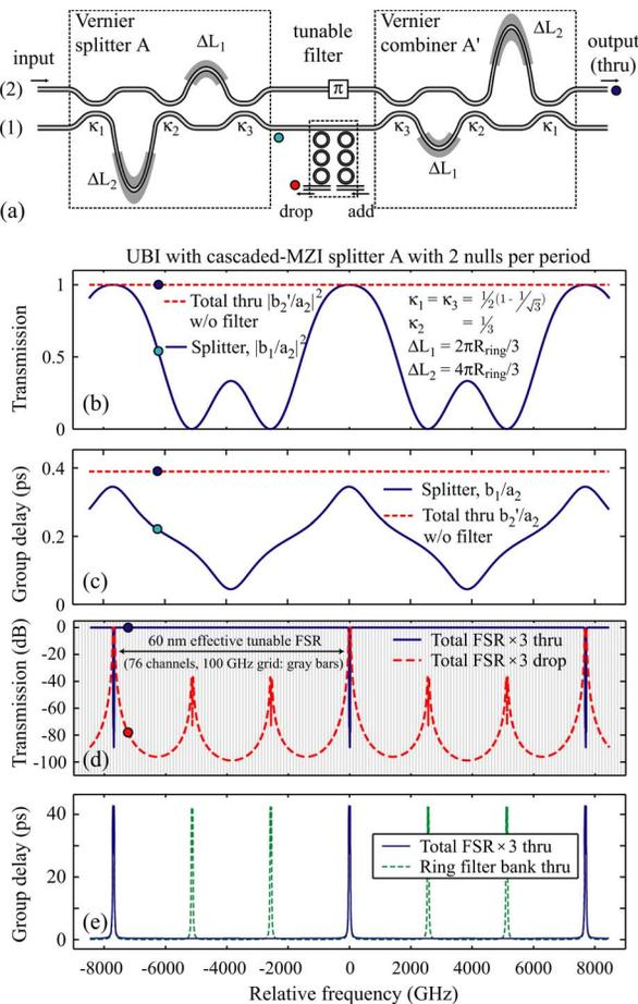
Fig. 3. (Color online) Nondispersive FSR multiplier ( $\times 3$ ) for an add-drop filter: (a) UBI with lattice-filter splitter/combiner and microring filter in one arm; (b), (c) splitter  $A$  and total output port amplitude and group delay responses without a ring filter show dispersionless broadband UBI operation; (d), (e) drop and output port responses with a filter show a small group delay at suppressed resonances.
