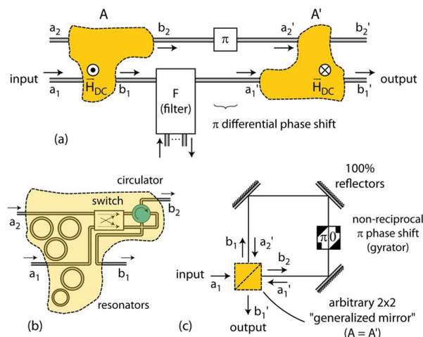
Fig. 1. (Color online) (a) General universally balanced interferometer, with a filter inserted in one arm. (b) Illustration of arbitrary splitting “mirror”  $A$  (may be nonreciprocal). (c) Folded UBI (requires a nonreciprocal  $\pi$  DPS).
