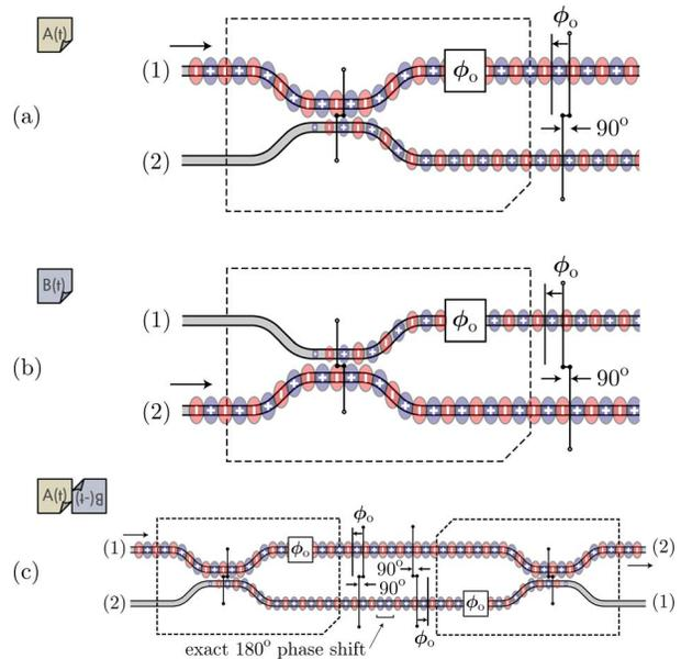
Fig. 2. (Color online) Canonical model of arbitrary LR four-port mirrors and constructed UBI. (a), (b) Excitation at port 1 or 2 gives  $\pi/2 \mp \phi_o$  phase; (c) cascading the splitter from (a) and the time-reversed and  $180^\circ$ -rotated version of (b) cancels arbitrary phase  $\phi_o$ . If the remaining broadband  $\pi$  phase shift is compensated for, a UBI is obtained.
