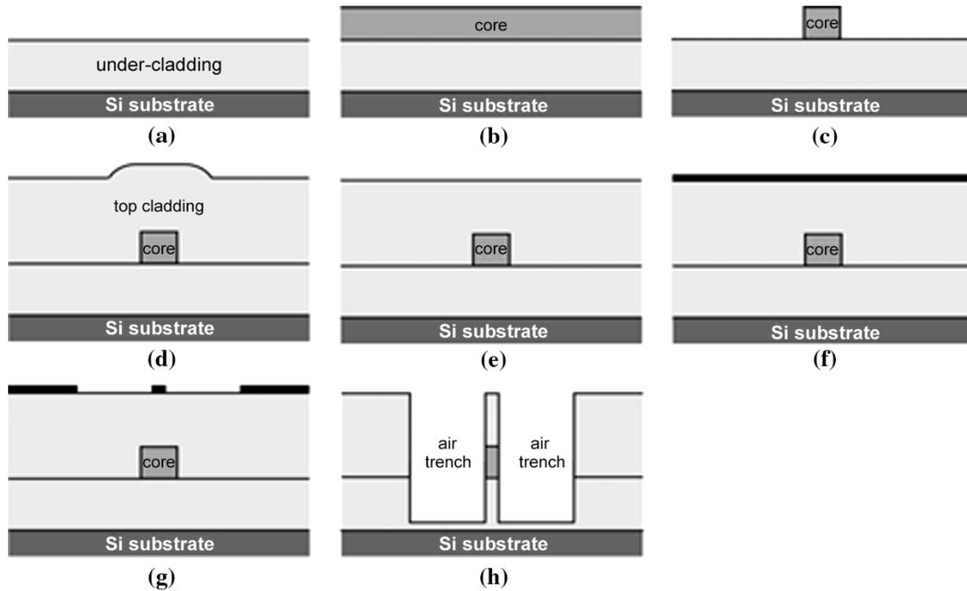
Fig. 3. Brief schematic of the ATB/T-splitter flow process (not to scale). All steps are done using conventional CMOS processes.
