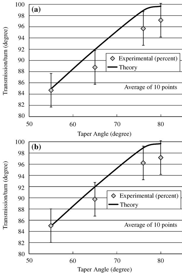
Fig. 7. Bending loss for ATB using (a) the TM mode and (b) the TE mode. Taper angle is varied from  $55^\circ$  to  $80^\circ$ . Experimental results are in good agreement with theoretical curves for transmission, as shown.
