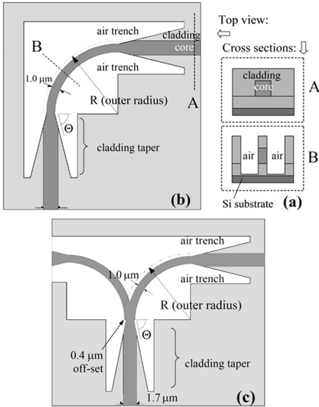
Fig. 1. Air trench design schematic. (a) Cross sectional view of (A) low index straight waveguide and (B) bend. (b) ATB. Outer radius = 3.7, 4.7, 6.2, 8.7, and 10.7  $\mu\text{m}$ , and  $\Theta = 55, 65, 76,$  and  $80^\circ$ . (c) Air trench T-splitter schematic.  $R = 10.7 \mu\text{m}$  and  $\Theta = 80^\circ$ .
