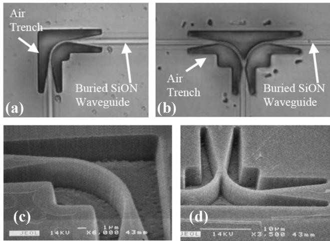
Fig. 5. Images of the fabricated structures. Optical microscope images: (a) AT bend and (b) T-splitter. SEM images: (c) AT bend (6000 $\times$ ) and (d) AT T-splitter (3500 $\times$ ).
