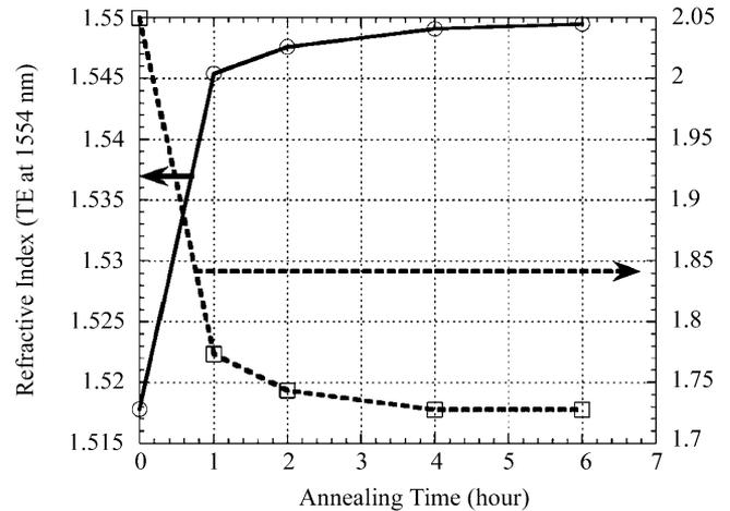
Fig. 4. Refractive index and thickness changes of the PECVD SiON after annealing (1554 nm TE mode). The refractive index increases by 0.033 and the thickness decreases by 15.7% as a result of consolidation annealing.
