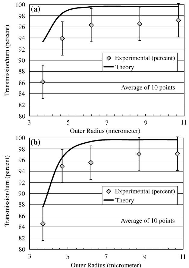
Fig. 6. Bending loss for ATB using (a) the TM mode and (b) the TE mode. Outer radii are varied from 3.7 to 10.7  $\mu\text{m}$ . The taper angle is fixed at 80°. Experimental results are in good agreement with theoretical curves for transmission, as shown.
