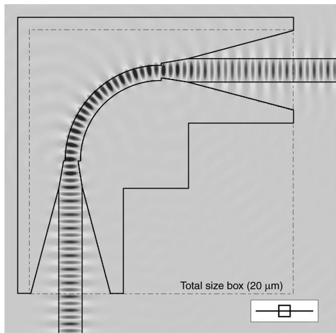
Fig. 7. Example C. Dominant electric-field plot from FDTD simulation. Total size box shown for reference (dash-dot square). The key in the lower right corner refers to transmission data in Fig. 8.
