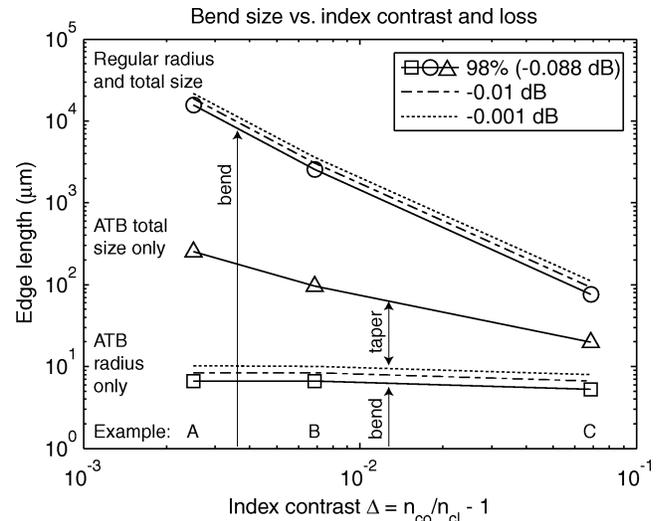
Fig. 4. Bend (radius and “total box”) size for regular waveguide bends and ATBs, showing improvement in size for the case of 0.1-dB loss. It is also shown that, on this scale of size variation, the relative change in radius is small for 0.01- and 0.001-dB loss.
