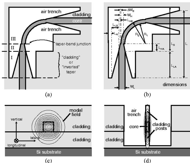
Fig. 1. ATB structure schematic: (a) Labeled plan view. (b) Dimensioned plan view. (c) Cross-sectional views in the low-index. (d) Air trench regions. Contour plots representative of the dominant modal electric-field component are superimposed on the cross sections (not to scale).
