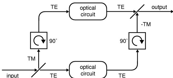
Fig. 2. Optical circuit layout for polarization-independent operation using polarization-dependent components and polarization splitters and rotators.
