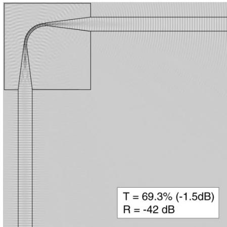
Fig. 9. The ATB from Example B without cladding tapers shows very poor performance. The core taper is virtually lossless, and the loss here is caused by the abrupt junction. No gain results if the core taper is lengthened.
