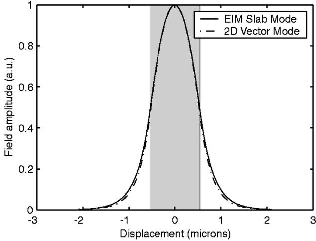
Fig. 11. Comparison of the dominant electric-field component distribution in the horizontal plane at the waveguide axis, as obtained from a vectorial mode solver (dash-dot) and as approximated using the EIM (solid). The EIM field is representative of the 2-D FDTD simulations.
