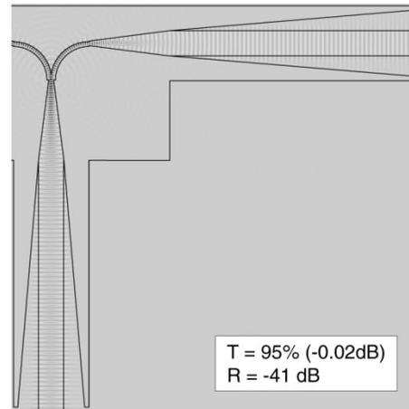
Fig. 14. Simple waveguide tee using ATBs (0.7% index contrast): Dominant  $E$ -field component plot from FDTD simulation. Transmission and reflection into source mode given in lower right corner.
