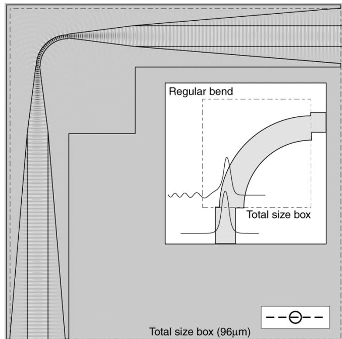
Fig. 6. Example B. Dominant electric-field plot from FDTD simulation. Total size box is outlined (dash-dot square) for ATB and for a regular bend (inset) for reference. Key in lower right corner refers to transmission data in Fig. 8.
