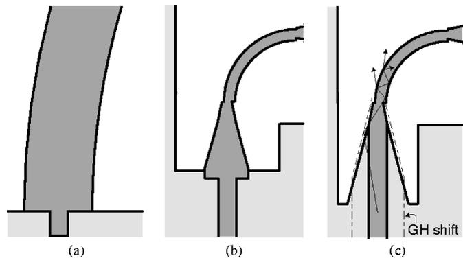
Fig. 3. Incorporating an air trench into a waveguide bend using (a) an abrupt junction, (b) an abrupt junction followed by a taper, and (c) the proposed adiabatic cladding taper. The bend radius is junction loss limited in (a), but curvature loss limited in (b) and (c). Junction loss is present in (a) and (b), but is virtually eliminated in (c). The dash-dot line in (c) shows a local Goos-Hänchen shift and a ray trace of coupling to the bend mode (not to scale).
