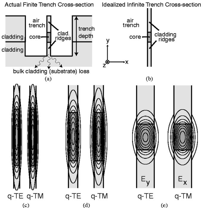
Fig. 10. Schematic of (a) actual air trench cross section and (b) the idealized trench, free of substrate loss. Fundamental quasi-TE and -TM modes of the ideal trench for Examples A–C are in (c)–(e), respectively. Mode plots are to scale individually, but not in proportion to each other. For an idea of relative scale, note that the waveguide width in each of (c)–(e) is the same.
