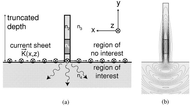
Fig. 12. Calculating substrate loss: (a) Setup of the 2-D equivalent current sheet method (ECSM). (b) Mode solver LM solution example: Real part of the  $E_y$  field component for the waveguide of Example B with the bulk cladding 0.6 core heights from the axis.
