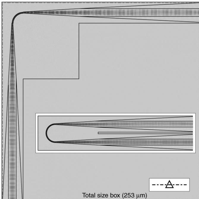
Fig. 5. Example A. Dominant electric-field plot from FDTD simulation, and the total size box (dash-dot square). Inset shows field plot of simulation used for throughput efficiency lower bound ( $180^\circ$  bend) due to simulation size constraints. Key in lower right corner refers to transmission data in Fig. 8.
