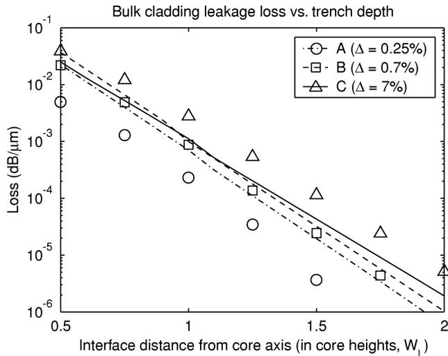
Fig. 13. Bulk cladding loss versus trench etching depth for waveguides of Examples A–C (Figs. 5–7) computed by approximate ECSM (lines) and numerical vector-field mode solver for leaky waveguides (symbols). The discrepancy is due to reflection at the interface with the bulk cladding, not accounted in the ECSM calculation.
