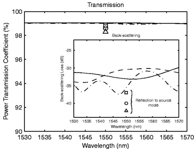
Fig. 8. Transmitted and backscattered power for cases A (dashed-dotted), B (dashed), and C (solid) through the output and input reference planes, respectively. True transmission and reflection into the fundamental mode is shown at the central wavelength (A-triangle, B-circle, C-square).
