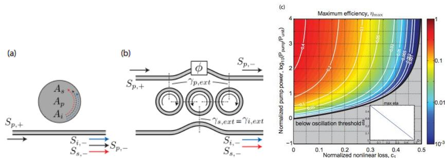
Figure 1: (a) Illustration of the micro-OPO model; (b) an example proposed multimode resonator based on 3 coupled microring cavities, showing an approach to unequal pump and signal/idler external coupling. (c) maximum efficiency vs. normalized pump power and nonlinear loss parameter with optimum OPO design.
