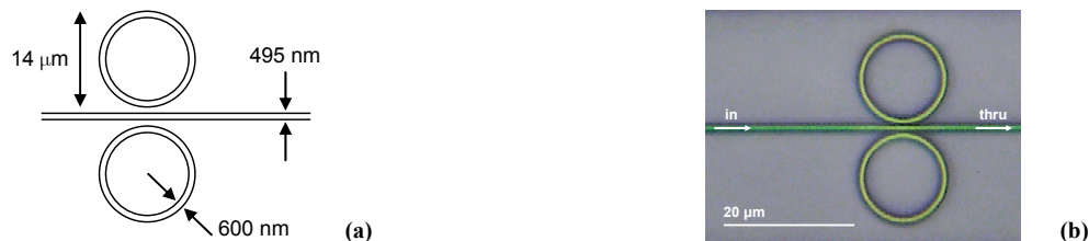
Fig. 1. Passive design of the interferometric dual-cavity slow light cell: (a) Illustration and dimensions, and (b) optical micrograph, before the fabrication of the titanium microheaters on top of the HSQ overcladding.
