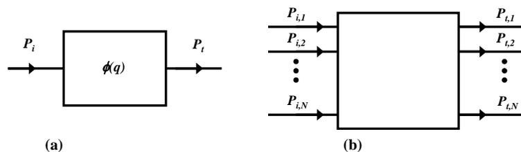
Fig. 1: (a) Lossless optomechanically variable dispersive element with one input and output (b) Lossless optomechanically variable multi-port system with N inputs and outputs
