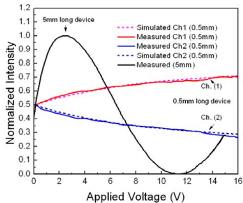
**Figure 2.** Measured and simulated normalized light transmission as a function of applied voltage.
