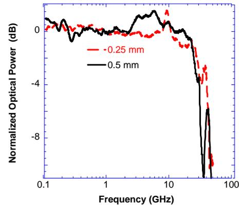
**Figure 3.** Measured frequency response of the modulator.
