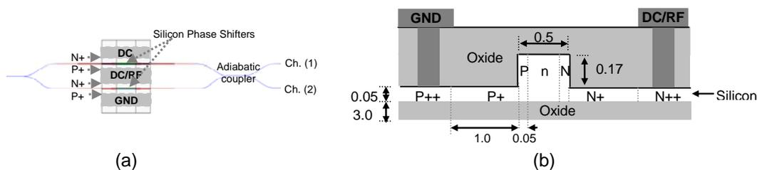
**Figure 1.** (a) Top-view layout of the dual-output modulator. (b) Schematic view of the cross-section of one of the phase shifters. (All dimensions are in  $\mu\text{m}$ ).
