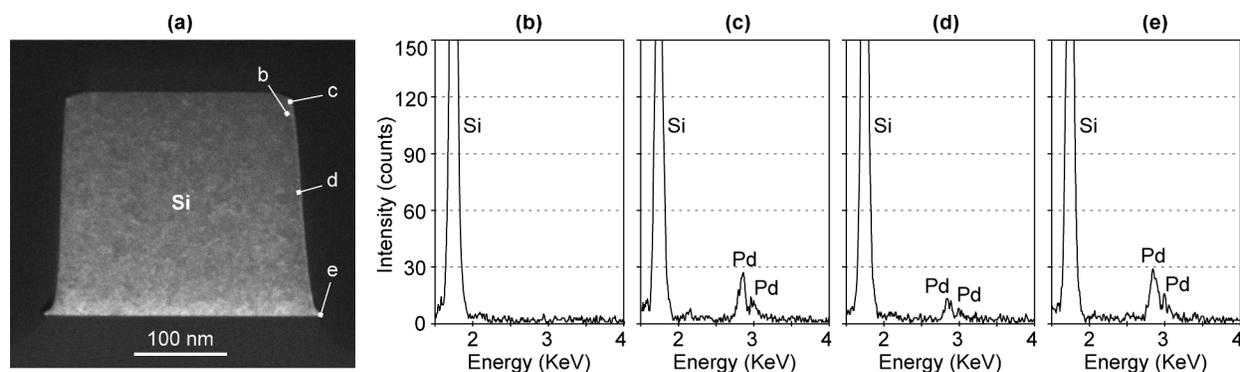
Fig. 2 STEM-EDS analysis of a Si waveguide etched in proximity of Pd and thoroughly cleaned with wet chemical processing. (a) Cross-sectional micrograph indicating where the EDS spectra were acquired. (b) EDS spectrum acquired 8-9 nm from the waveguide sidewall showing no detectable Pd. (c)-(e) EDS spectra acquired 1-2 nm from the waveguide sidewall showing the presence of Pd.
