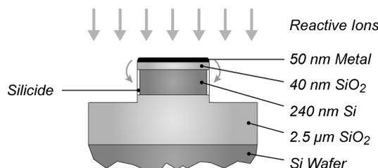
Fig. 1 Illustration of the mechanism to which the optical loss is attributed. At reactive-ion etching, sputtered metal atoms react with the silicon sidewall to form a silicide. The silicide is difficult to remove and induces an optical loss that is comparable to loss induced by a metal. The metal hardmask was thoroughly stripped before optical characterization.
