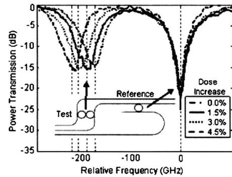
FIG. 2. Sample set of transmission spectra used for dose calibration experiments. Inset displays the device layout with a reference filter for each test filter. All frequencies are measured relative to the reference filter resonant frequency.
