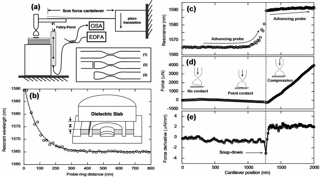
Fig. 1. (a) Tuning apparatus and (inset) probe fabrication process; (b) measured resonance wavelength of microring vs. distance of probe from ring surface (inset – schematic of tuning geometry); (c,d,e) resonance wavelength, force and force derivative vs. cantilever position.
