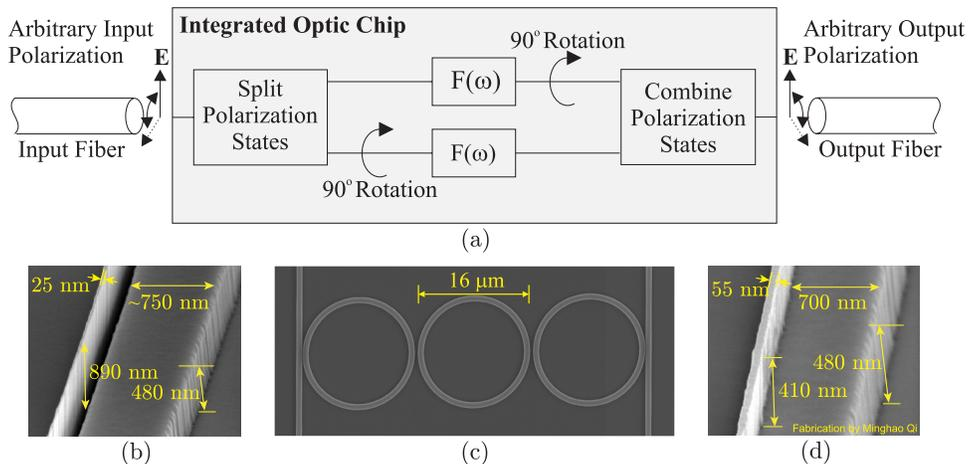
Fig. 1 (a) Diagram of an integrated polarization diversity scheme along with scanning electron micrographs of (b) an integrated optic polarization splitter, (c) micro-ring resonator, and (d) an integrated optic polarization rotator.
