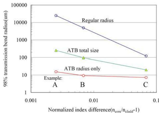
Fig.3. 98% transmission bend radius(R98) for conventional bend and air trench bend
