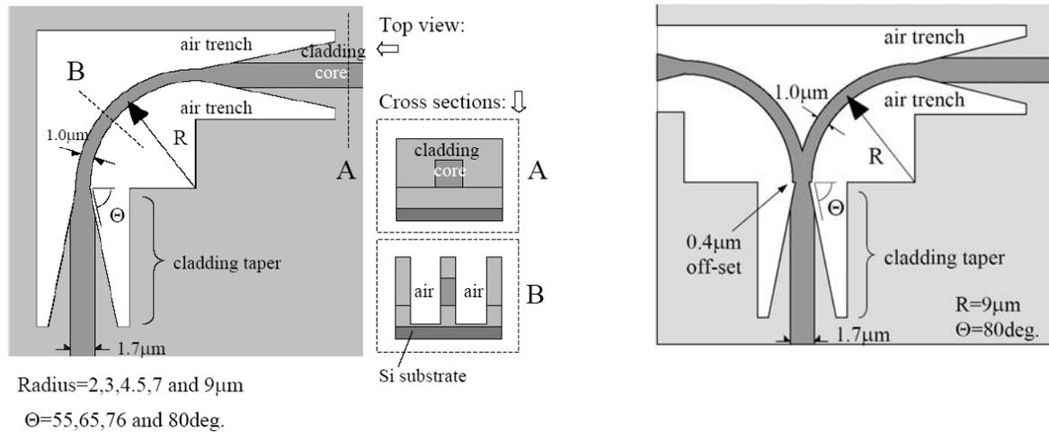
Fig.2a. (left): Air trench bend schematic – (A) Cross sectional view of low index (straight) waveguide, (B) Air trench region (bend)
