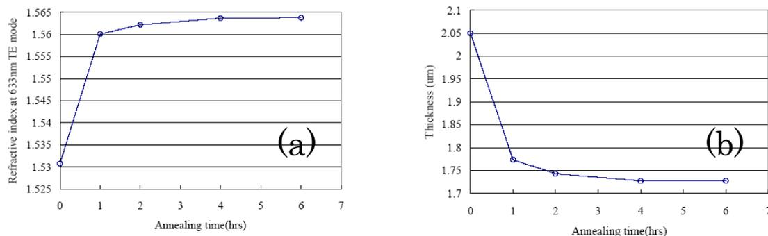
Fig.4. Properties' change during densification anneal, (a: left) Refractive index change, (b: right) Thickness change
