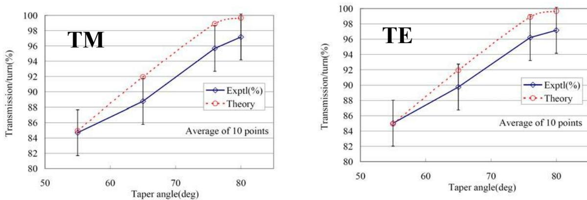
Fig.7. Bend losses for TM (left) and TE (right) modes. Taper angle is varied from 55 to 80deg. Radius is fixed at 9 $\mu$ m.
