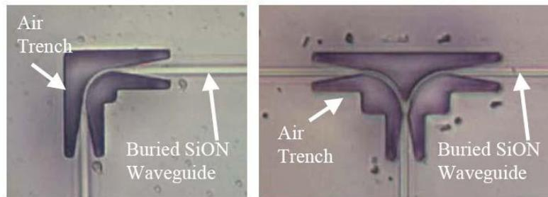
Fig.5. Optical microscope images for AT bend (left) and AT T-splitter (right)
