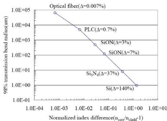
Fig. 1. 98% transmission bend radius( $R_{98}$ ) –Calculation is based on EIM method. Claddings are assumed to be silicon dioxide( $\text{SiO}_2$ )
