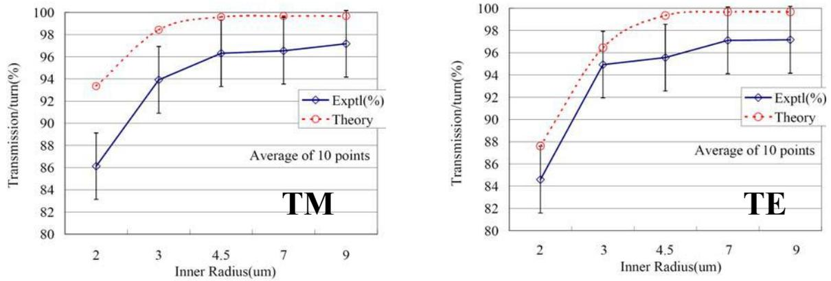
Fig.6. Bend Losses for TM (left) and TE (right) modes. Radii are varied from 2 to 9 $\mu$ m. Taper angle is fixed at 80deg.
