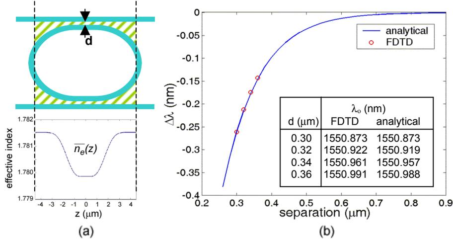
Fig. 1. Coupled-mode theory prediction and FDTD simulation of coupling-induced frequency shift. (a) geometry of CMT integration of the self-phase shift and effective index vs. position; (b) CIFS from coupled mode theory and FDTD.
