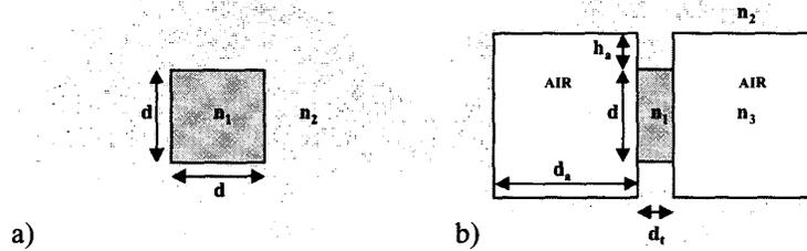
Fig. 1. Normal (a) and trench-flanked (b) waveguide cross-sections. Dimensions are  $d$  (width of low-index waveguide, and height of both),  $d_1$  (trench waveguide width),  $d_2$  (air trench region width), and  $h_2$  (extent of air trench above and below the waveguide).
