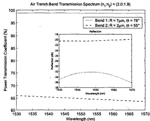
Fig. 3. Waveguide bend (left) with steep taper angle ( $55^\circ$ ) and small bend radius ( $2\mu\text{m}$ ). Poor taper performance between the high and low index sections shows multimode behaviour at the output and hence degraded throughput efficiency. Similarly to Fig. 2, a 50fs Gaussian pulse is seen in the field plot. Transmission and reflection spectra (right) are shown for this bend and the bend in Fig. 2.
