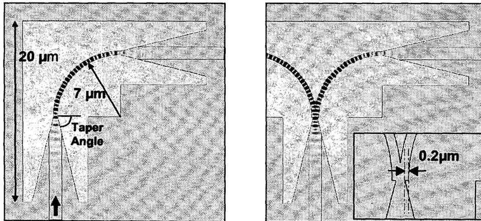
Fig. 2. Waveguide bend (left) and derived waveguide T-splitter (right). The electric field of a 50fs Gaussian pulse travelling through the bend clearly shows little radiation present in the turn. The inset on the right shows a waveguide step displacement ( $0.2 \mu\text{m}$ ) at the input of the T-splitter.
