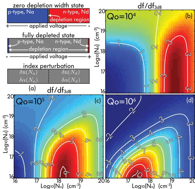
Fig. 4. (a) Simplified model for carrier-plasma modulator calculations. In the approximations used, the cavity goes from a negligibly small depletion width (top) to fully depleted (middle), which introduces a complex perturbation to the refractive index (bottom). Calculated resonance shift normalized to the total 3-dB linewidth for intrinsic quality factors (b)  $Q_o = 10^4$  (c)  $Q_o = 10^5$  (d)  $Q_o = 10^6$ .
