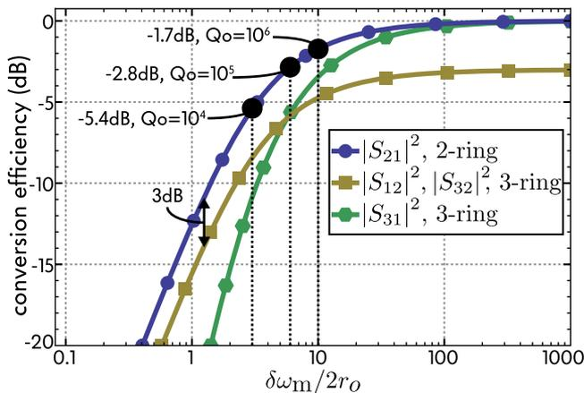
Fig. 2. Wavelength conversion efficiency as a function of modulation strength normalized to intrinsic bandwidth.
