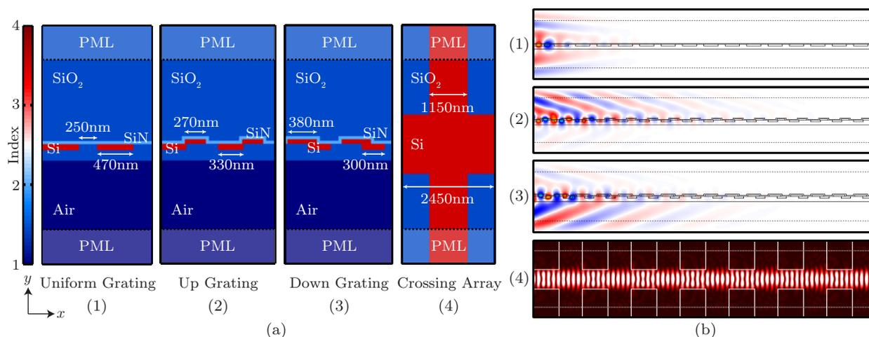
Fig. 1: (a) Two unit cells of (1) uniform, (2) upward, and (3) downward propagating grating couplers [1] and a unit cell of a (4) waveguide crossing array [4] showing index distributions and dimensions; (b) Bloch mode profiles at 1280 nm free-space wavelength of the gratings (1–3) and at 1200nm of the crossing array (4) simulated with PML boundaries in  $y$  and periodicity in  $x$ .
