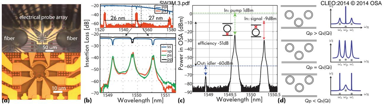
Fig. 2. **Four-wave mixing experiment in silicon 3-ring resonator:** (a) Micrographs of device under test with heaters; (b) optical transmission spectra of four port combinations (legend: “ps”=“pump bus” input, “signal bus” output) showing that signal (pump) bus couples weakly to pump (signal/idler) resonance; (c) seeded FWM with efficiency of  $-51$  dB; (d) Proposed orthogonal supermode linewidth engineering by controlling the “pump bus” and “signal bus” gaps.
