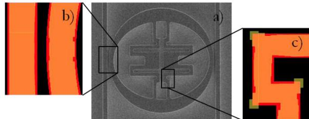
Fig. 1. (a) Planar micrograph of an example Adiabatic Ring Modulator (ARM) with integrated heater, drawn (red) and Optical Proximity Corrected (yellow) (b) waveguide to ring gap, and (c) local interconnect detail.
