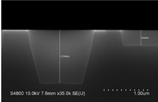
Fig. 2. Cross section micrograph showing adjacent Deep Trench Isolation (DTI) and Shallow Trench Isolation (STI). DTI enables fabrication of FEOL waveguides without undue coupling to the substrate, while the standard STI is used for the standard CMOS.
